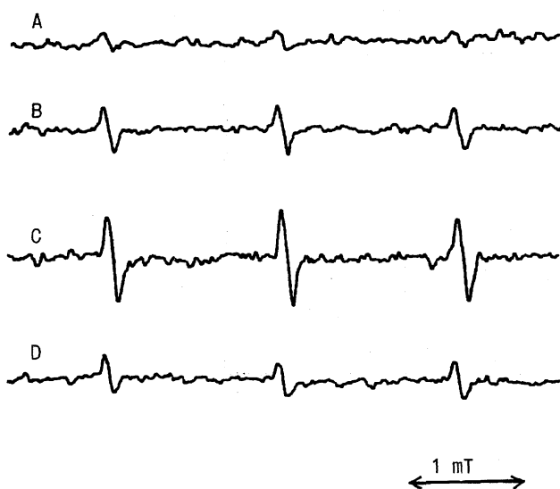
Fig. 11. ESR spectra of TEMPONE produced by irradiation of HP on the BH system. A: before irradiation, B: after 600-s irradiation, C: after 600-s irradiation containing 50% D 2 O, D: C + 1 mmol dm -3 NaN 3 .
